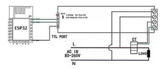
Fig 2. Connection of PZEM-004T and ESP32 unit
