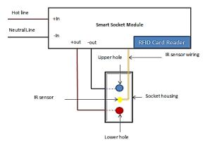
Fig. 4. The electrical connection of smart socket module for two holes of standard socket.
