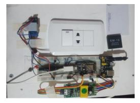
Figure 7: The main componentssmart socket module.
